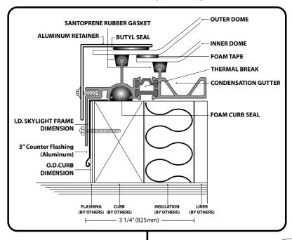
MAXIMUM OUTSIDE DIMENSION OF CURBS INCLUDING FLASHING AND ROOFING MEMBRANE
